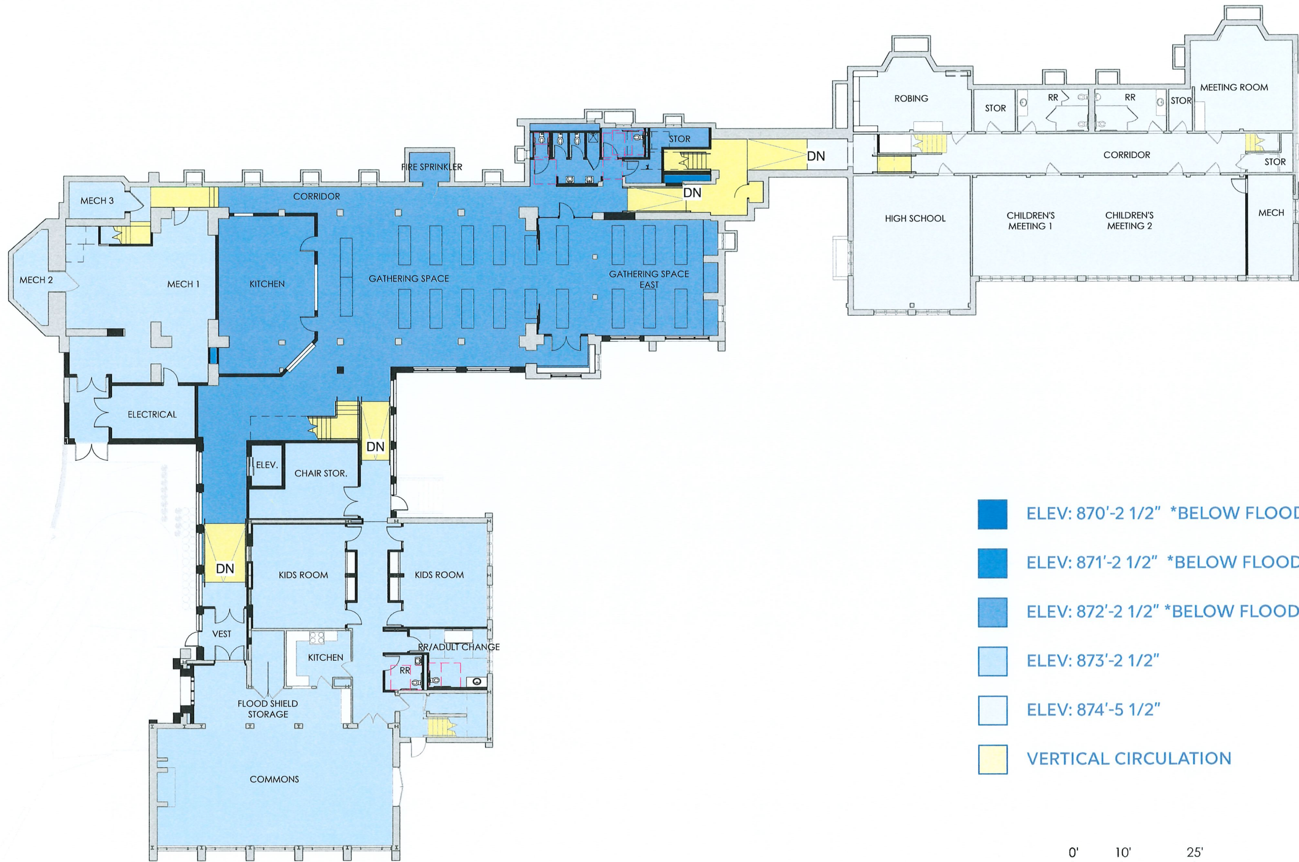
LOWER LEVEL FLOOR PLAN - MODIFIED FLOOR ELEVATIONS ST. STEPHEN'S EPISCOPAL CHURCH - ACCESSIBILITY AND SAFETY BETTERMENTS - VARIANCE REQUEST
